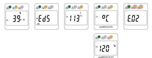
If different alarms occur simultaneously, the display changes at 3-second intervals. If several errors occur, the respective error codes are displayed alternately.
